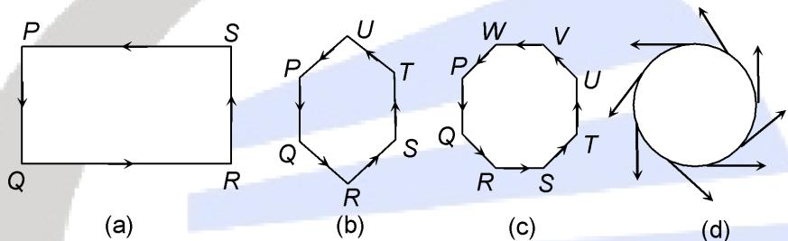
The force which is needed to make an object travel in a circular path is called **centripetal force**.
