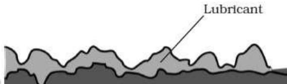
**Graphite:** Graphite is very soft and can be ground to a very fine state. It is then used as a lubricant in those parts of machinery, where oil cannot be applied.
