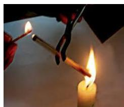
Observe that the flame appears at the end of the glass tube when a match stick is brought near it. This is due to the wax vapours that are coming out of the glass tube
