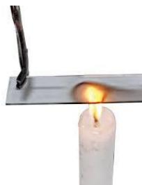
see that the portion of the copper wire just outside the flame gets red hot. It indicate that the non-luminous zone of the flame has a high temperature.
